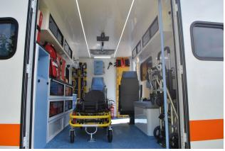
Near the bulkhead will be placed 1 vertical resin fittings complete of drawers and medical equipment Second vertical module to sink system compelte of pump, water basin, eternal plug for filling tank
